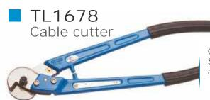
Cutter for steel cable (up to 16 mm) and steel rods (up to 10 mm). Small size (600 mm) and weight (2 kg), with titanium/aluminium arms. Interchangeable high quality steel blades.
