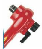
External ½" square drive. Inverter for right or left hand drive. Safe socket retaining system. Manufactured from chrome vanadium steel. Insulated and tested in accordance with EN60900.
